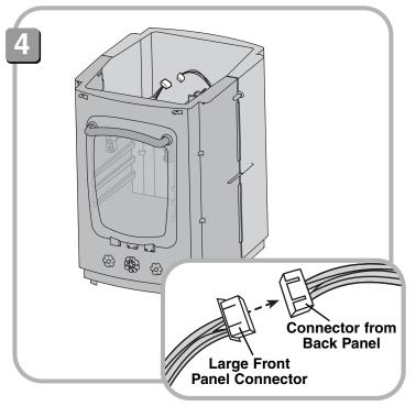
• Plug the large connector from the front panel into the connector from the back panel as shown.
